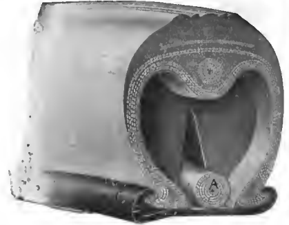
SECTION DAYTON AIRLESS TIRE.
